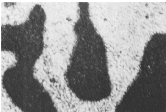
FIGURE 2A. Photomicrograph of DDA9M5,500 quenched to room temperature after 12 hours of annealing at 136°C. Magnification x 165.
